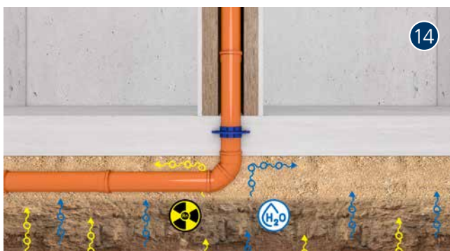
KGF110 set in concrete
