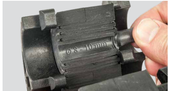
segments with exact diameter marking
