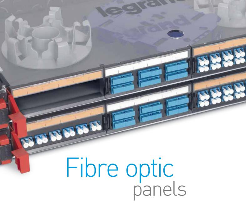
Completely renovated and redesigned fibre optic panels & drawers in high and very high density versions from 96 connectors per unit to 144 connectors per unit. Panels with sliding drawers and fast push-button system to facilitate upgrade and maintenance operations.
