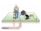
Find plastic pipe by tracing the push cable
