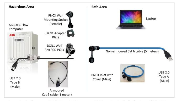
Customised cable comes with USB Type A & B connectors ATEX rated socket & plug for Ex-proof & Safe Zone.
