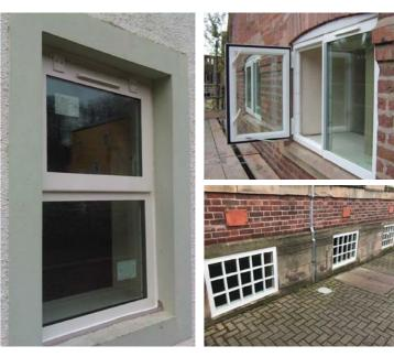
with an MMEngineering modified strong cockspur latch and a stainless steel casement stay for security closing, the opening light when closed and locked forms a fully watertight seal. Our flood defence windows are glazed with laminated safety glass panels assembled into double glazed K glass sealed units to comply with current building regulations.
